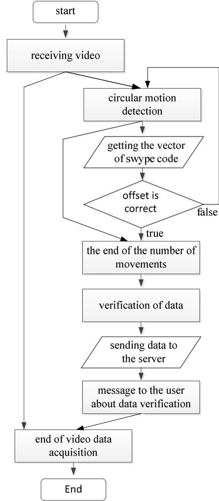
Figure 2. The verification algorithm with Swype code.
